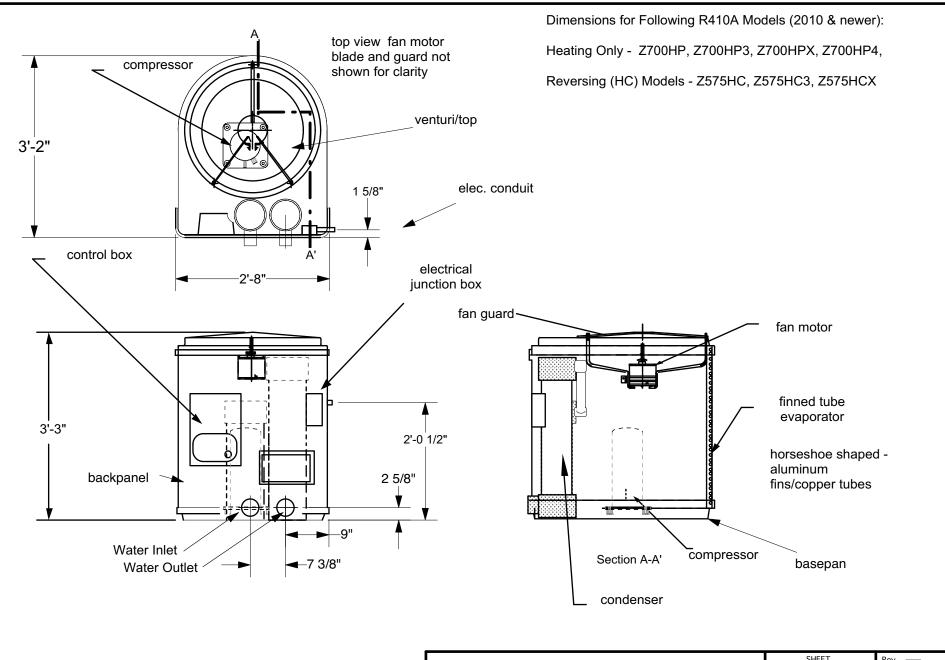
BOTH WATER INLET & OUTLET are Sch 40 PVC 1.5" Slip Fitting (ID) 2" MPT (OD)
